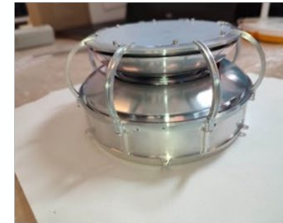
LEES sensor head prototype
